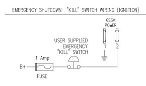
A single pole "kill switch" wired and installed by the user, stops the generator instantly in emergency situations such as a fuel spill. One switch pole (N.C.) kills power to the GSCM-mini opening all relays shutting down the ignition switch type generators.
