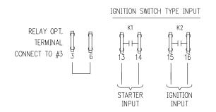
The K1 relay is used to switch the starter input which is looking for a momentary signal and opens when the generator has reached 35Hz. The K2 relay provides a continuous run signal for generators requiring a "maintained" ignition signal. When the GSCM-mini no longer receives a run command signal (terminal 5 or batteries fully charged, K2 relay opens telling the generator to shutdown. For GSCM-mini operational sequence details see Page 5, Section - 3
