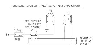
A double pole "kill switch" wired and installed by the user, stops the generator instantly in emergency situations such as a fuel spill. One switch pole (N.C.) kills power to the GSCM-mini opening all relays. The other switch pole (N.O.) shorts out the magneto for an instant stop.
