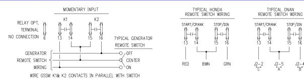
The K1 relay is used to switch the start/crank input which is looking for a momentary signal and opens when the generator has reached 50Hz, or half speed. The K2 relay provides a momentary "stop" signal until the generator AC Hz has dropped to zero. For GSCM-mini operational sequence details see Page 4, Section - 1
